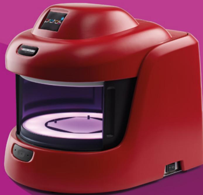
**aCOLyte 3** is an affordable, automated colony counting device. The system is available in one configuration and has simple-to-use software and lighting from white LEDs above and below your plate. These features allow you to automatically count colonies on a range of pour and spiral plate media and then directly transfer your results to Excel or Open office. The system also has a detachable screen for eliminating strong ambient light, if it causes plate reading issues in your laboratory.
